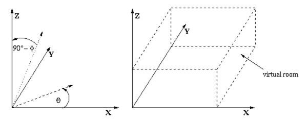
The <u>reflection coefficients</u> of the walls can be given in the range from 0.0 to 1.0, where a coefficient of 1 means total reflection a 0 total absorbtion. Thus you can omit a wall by setting its coefficient to zero. To simulate a surrounding with just a floor, set all coefficients except that of the floor to zero.
